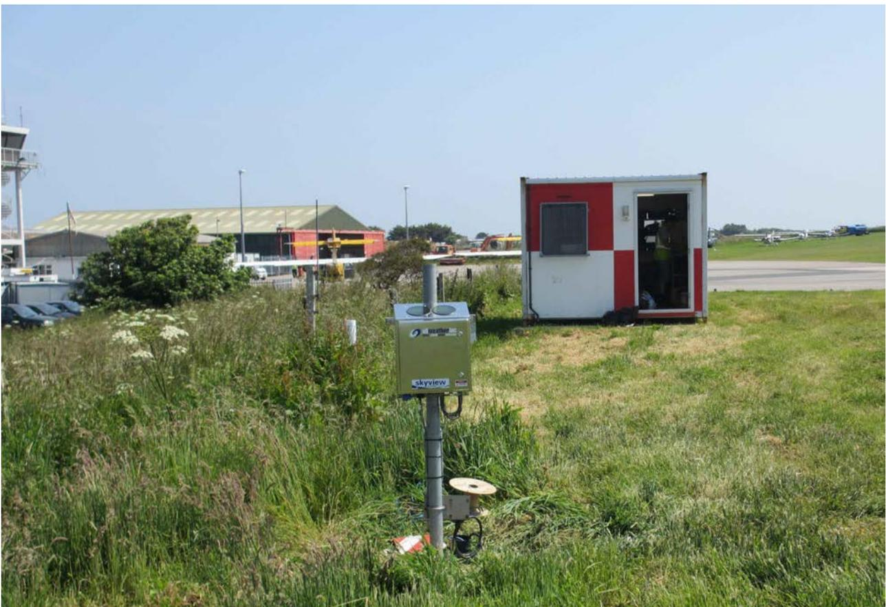
*The new Alderney Airport laser ceilometer is installed - the instrument is capable of measuring cloud base heights up to 24,000 feet above the airfield.*
