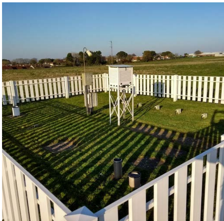
Temperatures are still measured in a Stevenson Screen at a height of 1.25m above the ground and situated to the north of the runway in a purpose built meteorological garden.
